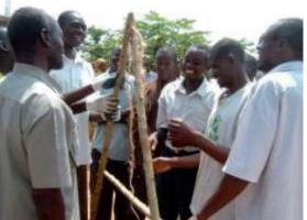
Measure the middle point on each stick and nail the cross bar across the two. Make it relative to one's size. Make a middle point on the cross bar, tie the string from the top onto the heavy object. The string must pass through the middle point – if it doesn't you have not made it properly. Make your contours using the A frame.
