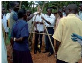
Keeping one leg of the A frame on the floor, move the other leg round along your plot. When the string passes through the middle point, mark where the  $2^{nd}$  leg is. Then keep that leg on the floor, and move the first leg of the A frame around. When the string passes through the middle point, mark again. And so on..... You will soon end up with a row of markers
